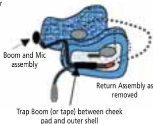
When replacing the cheek pads, trap the boom between the outer shell and the inner cheek pads plastic tongue if it has one. Tape or glue if required. **Do not modify the helmet.**
