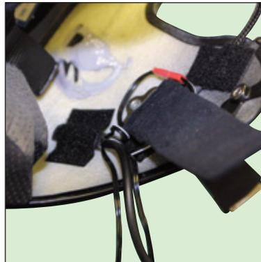
Velcro the 7-pin loom to the inner shell behind the chin strap.
