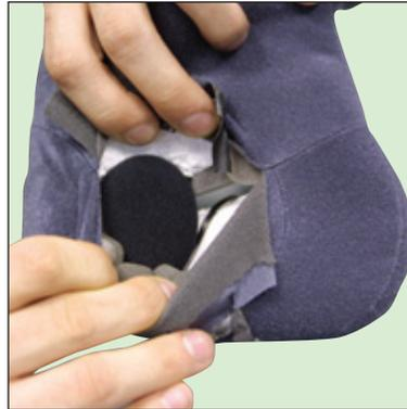
Place a small strip of velcro where the circle is. The speaker is then placed in the cheek pad in a vertical position with the wire to the bottom of the speaker. The wire is then placed through the chin strap hole. The fabric is put back in place and taped back up in its original state.
