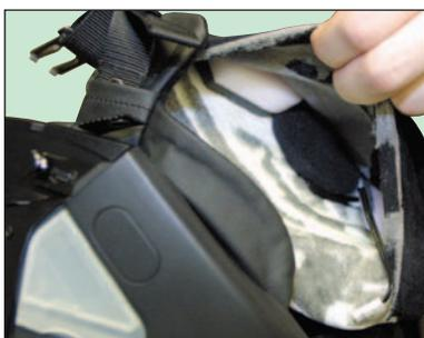
**4** Place a strip of loop velcro over the hole. Place the speaker over the moulded hole onto the velcro with the speaker in a horizontal position and the wire coming from the back of the speaker. Replace the liner to its original position.
