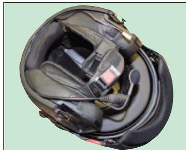
**8** Repeat the same to the other cheek pad so you have both speakers inside the liner of the cheek pads. Carefully tidy up the longer wire remaining around the back of the helmet and then connect the last white connector together so both speakers are connected.
