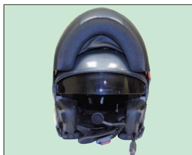
**10** Finally, make sure that you can easily flip the black visor up and down, if not you may have to adjust the loom so the visor works as should.
