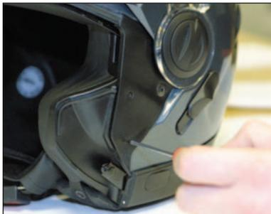
**1** Firstly, remove the horseshoe shaped padding on the bottom of the helmet by un-clipping the two press-studs. Remove the two T8 Torx screws on the side of the helmet as shown. These hold the cheek pads to the helmets outer shell.
