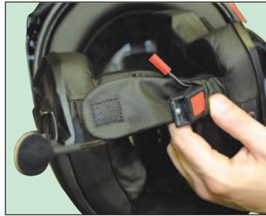
**5** The microphone boom needs to be placed up where the strap comes through the cheek pad leaving just a sufficient amount of microphone to reach the centre of your mouth.
