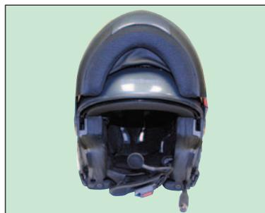
**9** Once the connectors are all connected together and the wires are tidily tucked away, put the horseshoe shaped padding back on the base of the helmet.
