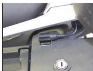
The passenger lead comes out near where the passenger sits and is positioned on the plastic near to the panniers.
