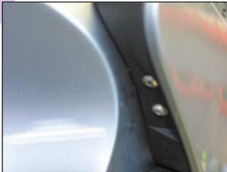
Remove the x2 T25 screws holding left hand side dash in position and the two other screws on top of the dash.
