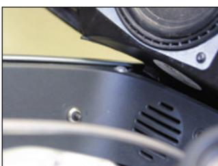
Drill 6.5mm hole around or near the audio controls and fit the toggle switch.
