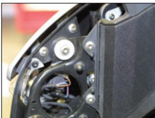
Remove the x3 T25 screws holding each of the speakers in position.
