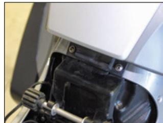
Remove the x2 T25 screws in the middle of the tank.
