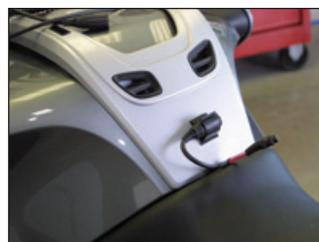
The riders lead follows the chassis down towards the tank and finishes between the tank and the riders seating area.
