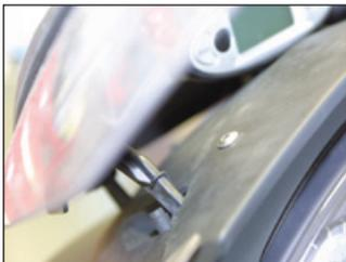
Remove the x2 T25 screws from the fairing where the top fairing and bottom fairing are joined.
