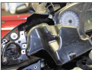
Pull out speakers to expose speaker wires behind.
