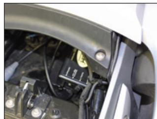
To bike power the Autocom unit, take the earth and the 12 volt positive from the auxiliary power socket towards the rear of the bike. Do not use the socket itself, but strip into the two wires at the back of the socket. The 12 volt positive wire is the red and green wire, the negative earth wire is the brown.
