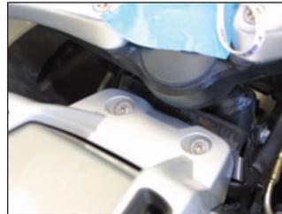
Remove the x4 T25 screws holding the tang bag holder in place.
